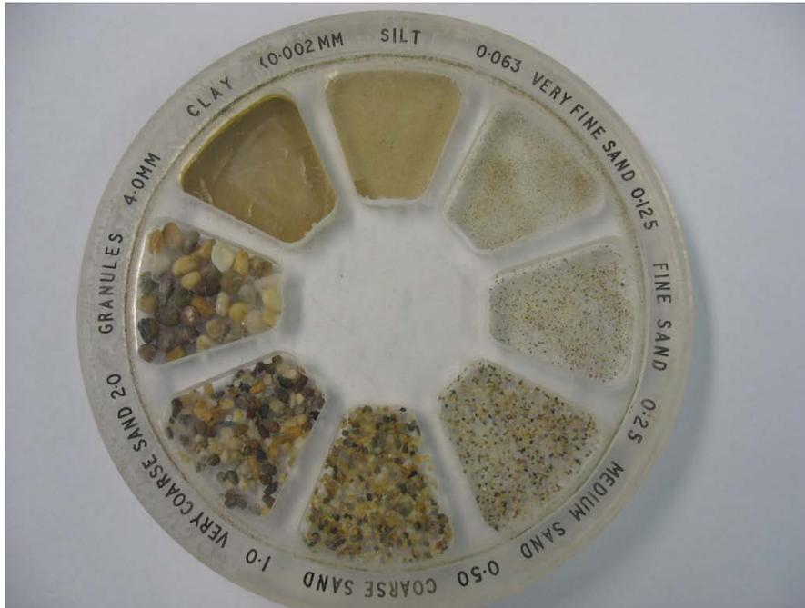
**Figure 2:** Sediment sizing wheel
