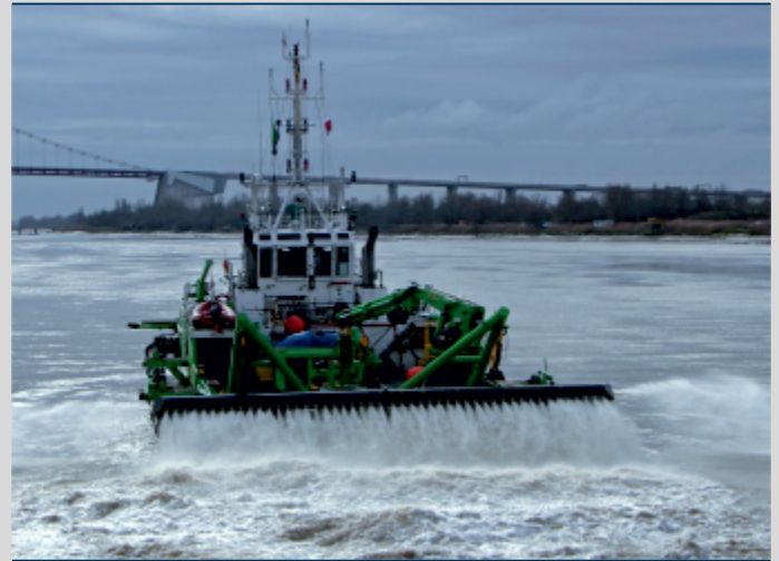
Water injection dredging (source: DEME)
