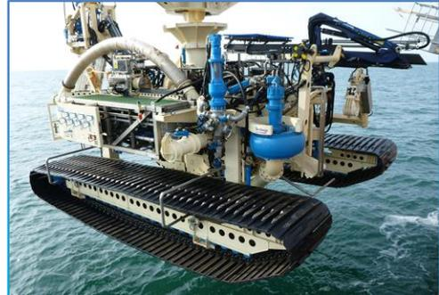
Expected progress rates of the vehicle are to be determined to make a more realistic assessment of the expected project durations in the pre-execution stages. This can only be done if specific knowledge regarding the interaction between seabed soils and track drive is available. Further-more it is interesting to look at the most optimal setup of the vehicle for each project, make the machine work more efficiently and decrease the trenching duration.
