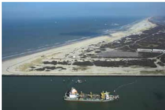
*Beach nourishment for a dune compensation project on the Delfland Coast, the Netherlands. Sand is pumped to site through a pipeline crossing the 'Van Dixhoorn triangle', a land reclamation near Port of Rotterdam.*
