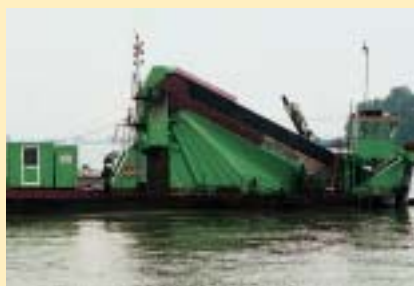
The encapsulated bucket dredger (above) and the auger dredger (left) are two examples of specially designed environmental dredging equipment.
