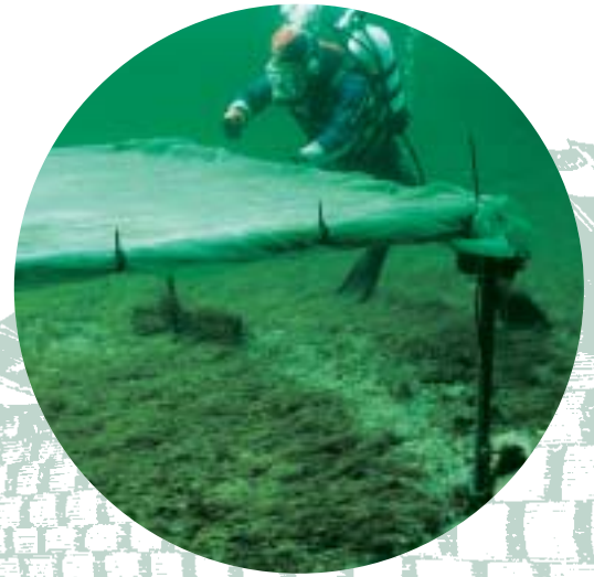
During dredging for the Øresund Link between Denmark and Sweden, scuba divers take samples of eelgrass every other week to assess impacts.
